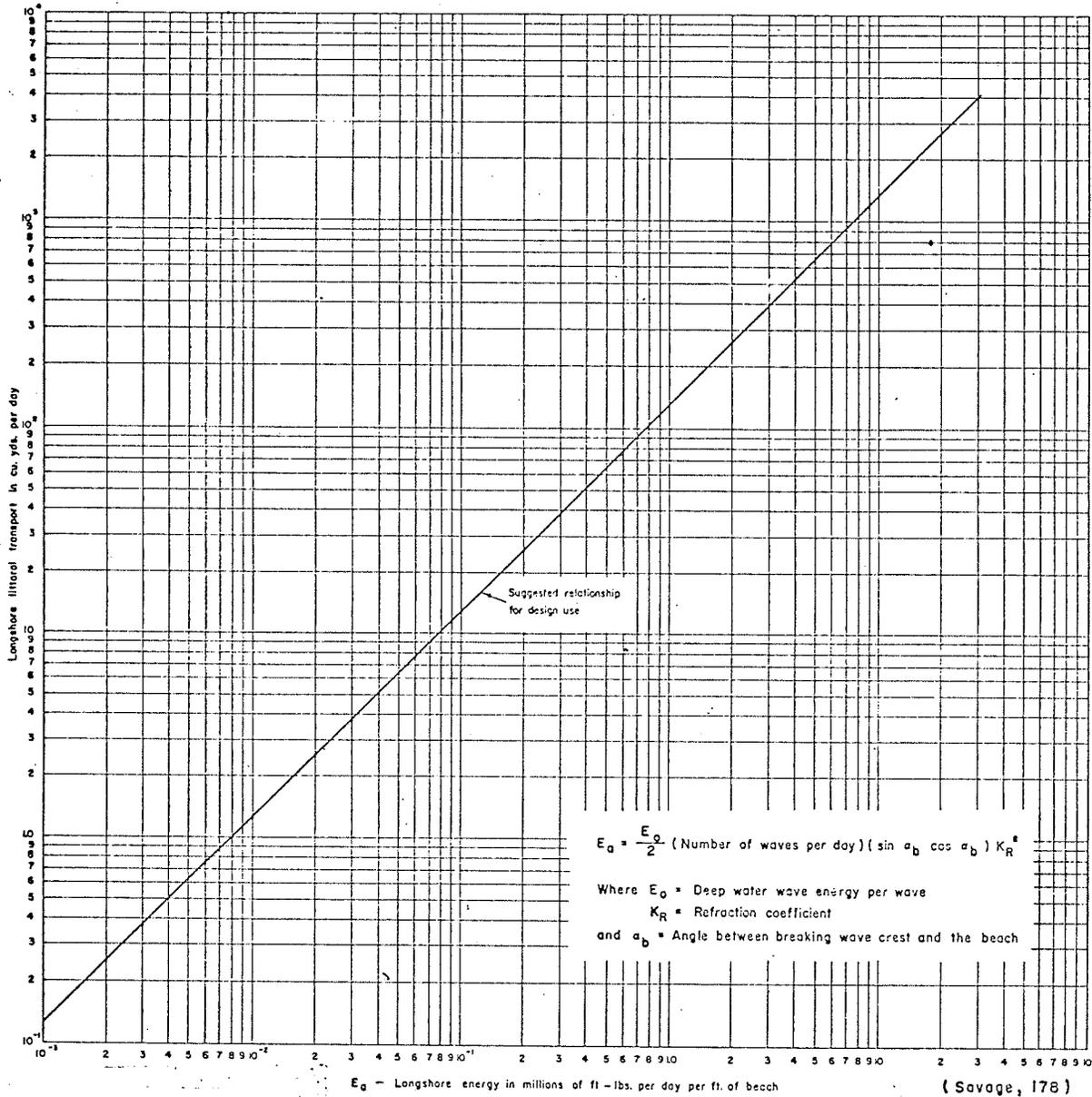
RELATION BETWEEN LONGSHORE COMPONENT OF WAVE ENERGY AND LITTORAL TRANSPORT RATE
